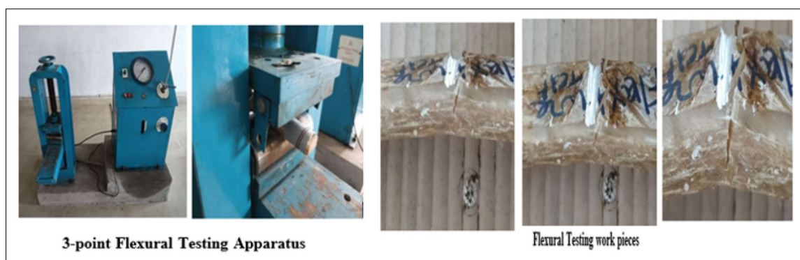
Figure 3: 3-Point Flexural Testing
